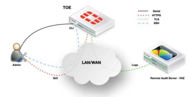
Figure 1: TOE Architecture
